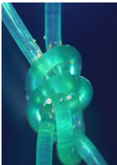
Figur 7. Bionedbrydelige materiale (polybutylene succinate co-adipate-co-terephthalate PBSAT) til garnfiskeri © DTU Aqua / DTU Sustain.
