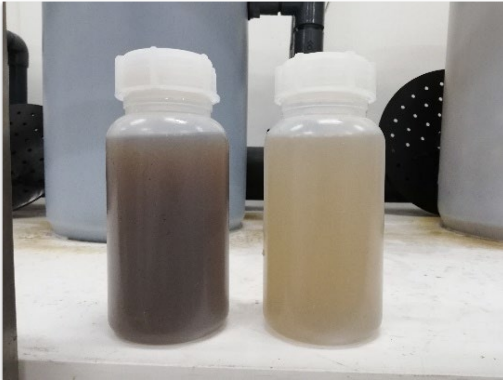
Figure 7-6. Representative subsamples of reject water (20-23 L) based on squeezing organic loaded from foam biofilters with low HRT (left) and high HRT (right). Photo by Bence Dániel Kovács.
