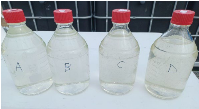
Figure 5-21. Water samples were collected at the experiment site for molecular analysis. The water samples were transported, filtered, and treated on the same day in the laboratories of DTU Aqua, Lyngby.
