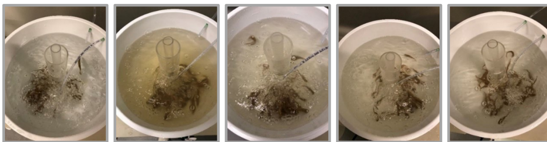
Figure 6-1. Experimental tanks exposed to organic waste material (foam fraction). From left to right: control tank, 1:3, 1:6, 1:12, 1:24 foam to water ratio exposed tanks.
