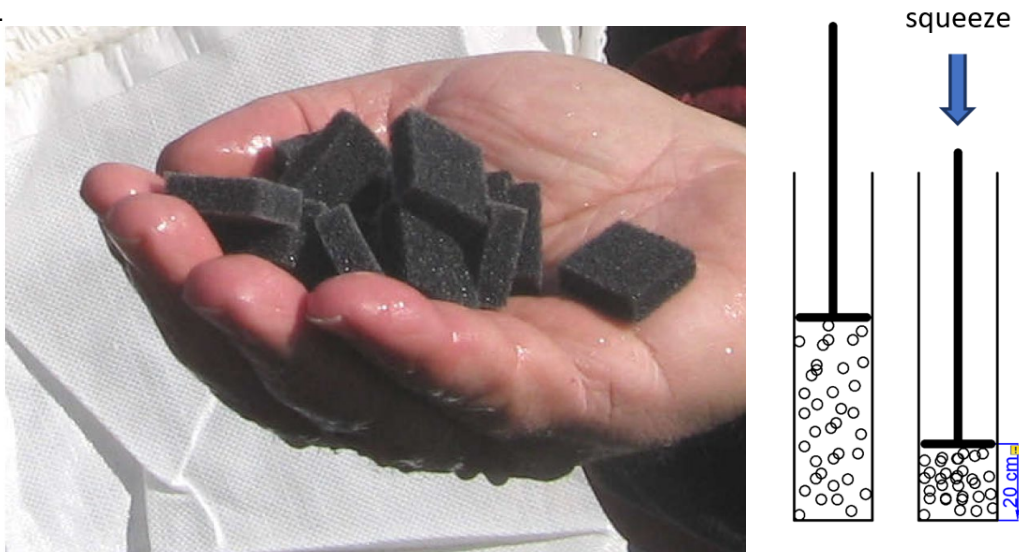
Figure 7-3. Picture of Levapor bioelements, and a sketch of the principle of standardized backwashing/squeezing the bioelements to extract collected organic matter.
