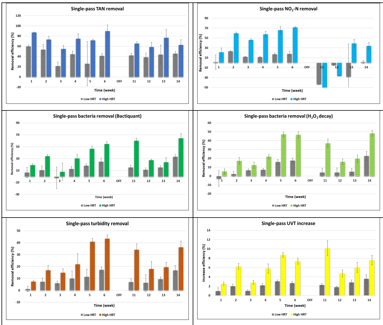
Figure 7-4. Results of removal efficiency of fixed bed bioreactors with Levapor foam. The removal efficiencies (RE) are calculated as ([Inlet]-[Outlet]) \times 100/[Inlet] and reflect average \pm sd (N=4). The reactors were operated with 400 l/h, ~ 2.4 min hydraulic retention time [Low HRT] or 60 L/h ~ 14 min HRT [High HRT]. A) Total ammonium N, B) Nitrite-N, C) BactiQuant, D) H 2 O 2 decay assay, E) Turbidity, and F) UVT.
