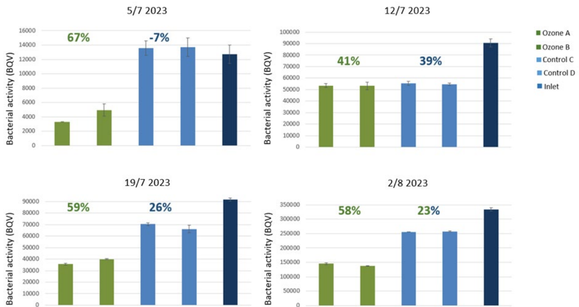
Figure 5-12. Microbial activity based on Bactiquant measurements at five different sampling points and four sampling times. The bars show the average \pm sd of samples collected and fixed at 08:30, 09:30 and 10:30.
