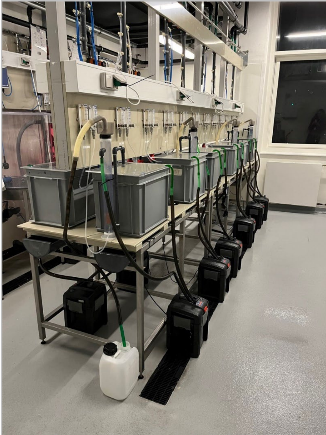
Figure 6-6. Experimental set-up in the high containment infection facilities in DTU Aqua, Lyngby. Each 30 L tank was individually recirculated (biofilters can be seen on the floor for each tank). On the foreground, one of the tanks treated with foam fractionation is shown: the water from the biofilter is directed towards the protein skimmer device, where foam is created and overflowed to a separate reservoir (white tank on the floor). The water fraction from the protein skimmer is instead redirected to the main tank.
