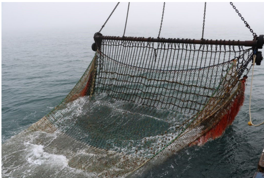
Figure 4.1. The beam trawl rigged chain mats used in the BACI experiments on circalittoral mixed sediment in the Jammer Bay.
